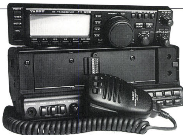
The Yaesu FT-900 h.f. transceiver with the demountable front panel detached. The model reviewed by Rob Mannion G3XFD was supplied with the optional automatic a.t.u. unit (transceiver designation FT-900AT) and the optional 'quick release' mounting unit for the control, with associated remote control cable.
